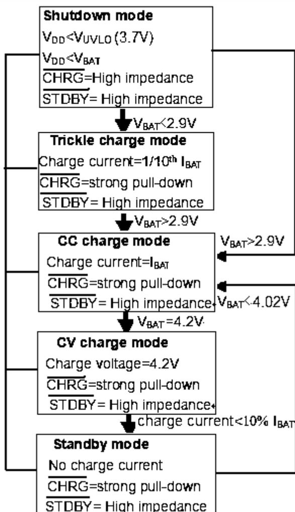
Fig.1 State diagram of a typical charge cycle
